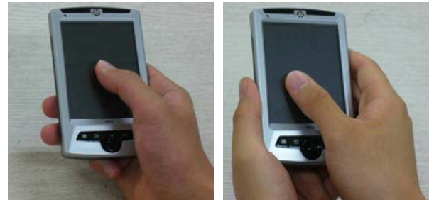
Figure 2. Two methods to hold a PDA. Left and Right figures showed one-hand and two-hands holding, respectively.
